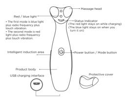
Long press the power button 2S to turn on/off.
